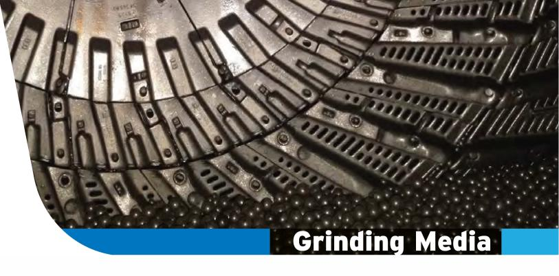
ME Elecmetal designs, manufactures and supplies premium quality forged steel grinding media for SAG and ball mills.
