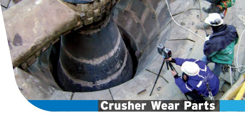
Wear components for crushing processes are subjected to severe impact and high abrasion, requiring solutions made from high strength and abrasion resistant alloys.
