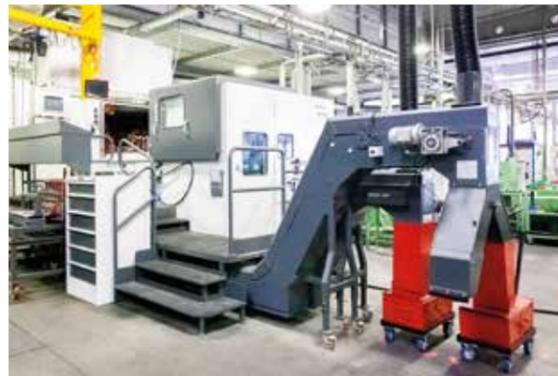
In addition to the standard products, we also offer you special custom solutions - such as the HEICO-LOCK® Combi Bolt or HEICO-LOCK® Special Washers. In order to be able to respond quickly and flexibly to your wishes, we have modern machinery at our disposal. On high-performance multi-stage presses, such as the SACMA SP 470, we are able to produce cold forged parts according to customers' drawings using cold forming or warm forming methods.
