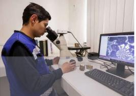
• Metallurgical laboratory for verification of microstructure and heat treatment control.
